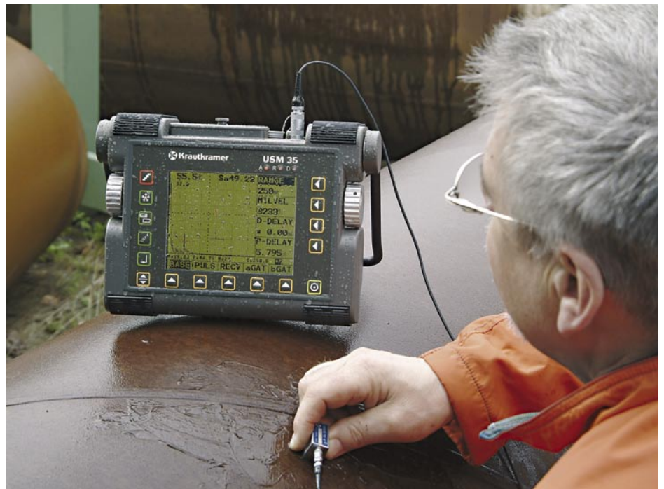
Inspection of a weld
