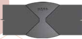
30 Porosity in Double Vee (sub-surface) UT, RT
