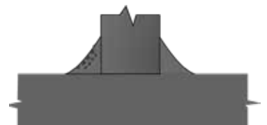
33 Porosity in Fillet (surface breaking) VT, MT/PT
