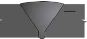
50 Lamination in Single Vee (base metal) UT
