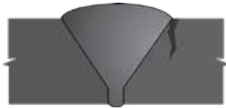
10 Toe Crack in Single Vee MT/PT, UT
