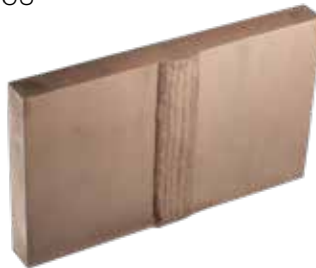
WELDED PLATE 1.0"x6"x10" #P108
