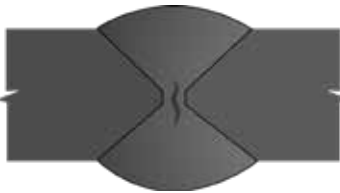
15 Centerline Crack in Single Vee (sub-surface) UT, RT
