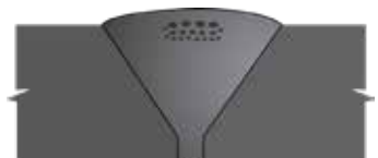
30 Porosity in Single Vee (sub-surface) UT, RT
