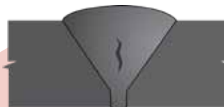
15 Centerline Crack, Single Vee (sub-surface) UT, RT
