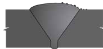
90 Weld Splatter on Single Vee, VT, RT
