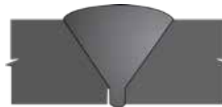
55 Lack of Fusion in Single Vee (surface breaking at root) MT/PT, UT
