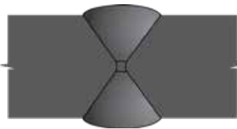
57 Incomplete Root Penetration in Double Vee, UT, RT
