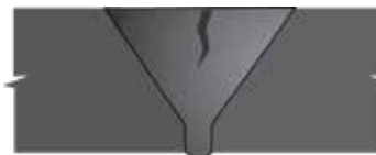
16 Circumferential Crack in Single Vee, flush crown MT/PT, UT
