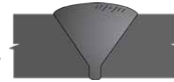
92 Chipping Hammer Marks on Single Vee, VT, RT
