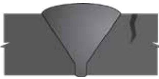
18 Base Metal Crack in Single Vee (top HAZ area) MT/PT, UT
