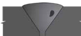
37 Slag Inclusion in Single Vee (weld groove area) UT, RT
