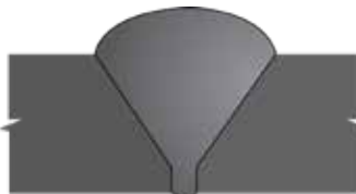
74 Excess Crown in Single Vee, VT
