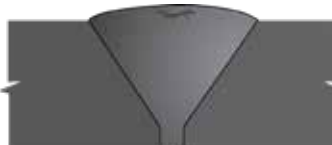
20 Crater Crack (crown stop-start area) MT/PT, UT
