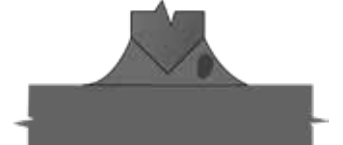
38 Slag Inclusion in Fillet (root area) UT, RT
