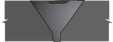
17 Transverse Crack in Single Vee, flush crown MT/PT, UT
