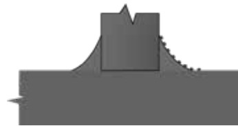
91 Weld Splatter on Filler VT, RT
