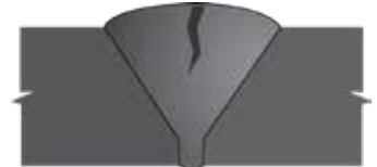
14 Centerline Crack, Single Vee (surface breaking) MT/PT, UT, RT
