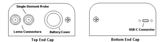
The top end cap is where all connections are made to the **ZX6**. The diagram above shows the layout and description of the connectors:
