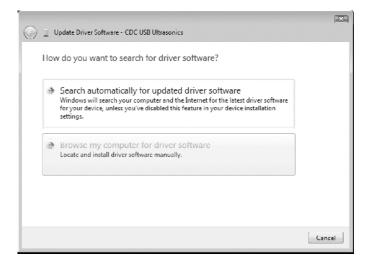
Select "browse my computer" and navigate to the directory where the driver was saved on your PC and install the driver. When the installation is completed, the following window will be displayed:
