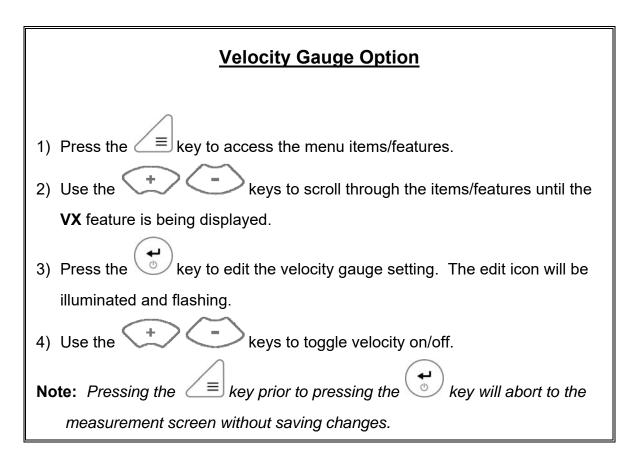
5) When the desired **VX** setting is displayed, press the key to set the status and return to the measurement screen.
