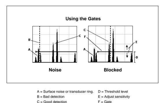
**<u>Start:</u>** This feature is only available to gate 1 and determines where the gate will start in terms of thickness. For example, if there's a great deal of noise from the initial pulse, or in the material, the gate can be set further out in time/thickness to avoid and block the noise from being detected.
