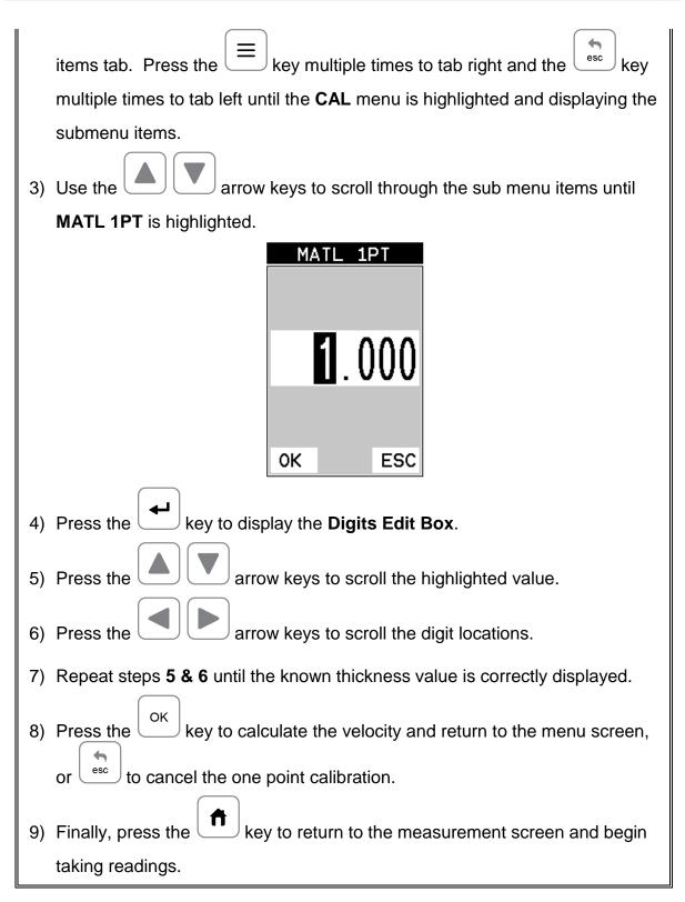
Note: CHECK YOUR CALIBRATION! Place the transducer back on the
