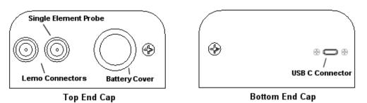
The top & bottom end panels are where all connections are made to the *MX2-DL*. The diagram above shows the layout and description of the connectors:
