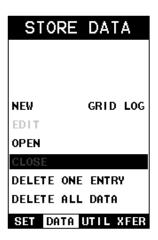
3) Press the key to close the active file. **Note:** Following the key press, the **CLOSE** text will be grayed out indicating the file has been close and is no longer active.
