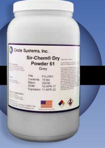
Sir-Chem<sup>®</sup> Dry Powder 61 is a highly refined nonfluorescent grey magnetic powder used for dry method magnetic particle inspection. It is designed to be used in visible light to reveal minute discontinuities on fabricated components or weldments such as bridges, pipes, large tanks, machinery and equipment.
