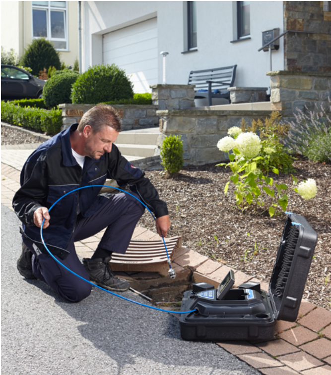
The robust color camera head is waterproof to IP 67 rating. With a diameter of just 1.5" it easily negotiates bends in pipes of 2.5" and larger.
