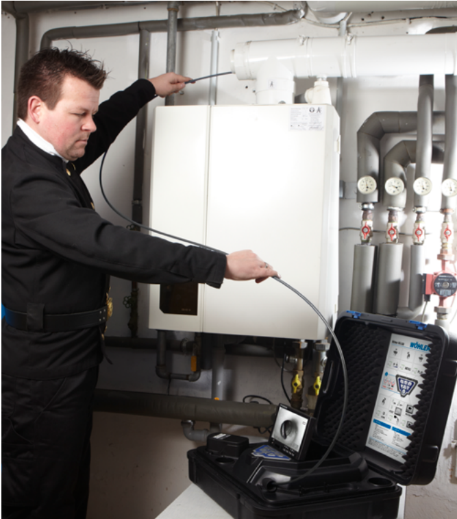
The 360° pan- and 180° tiltable color camera head easily negotiates 90° bends.
