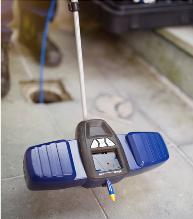
The Wohler L 200 Locator makes it possible to locate the camera head wirelessly.
