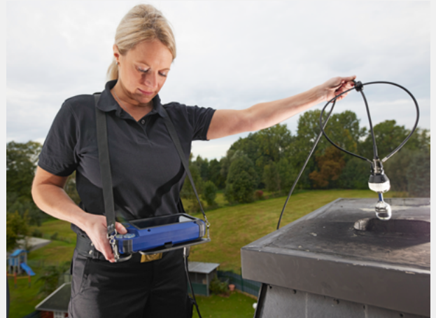
Cable camera: Perfect for inspections from the roof.
