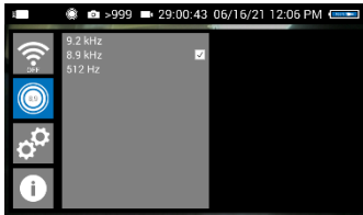
Fig. 29: Locator detection with 8.9 kHz transmission frequency selected
