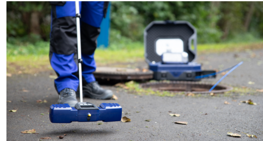
With the Wohler L 200 Locator, the camera head can be located with pinpoint accuracy.
