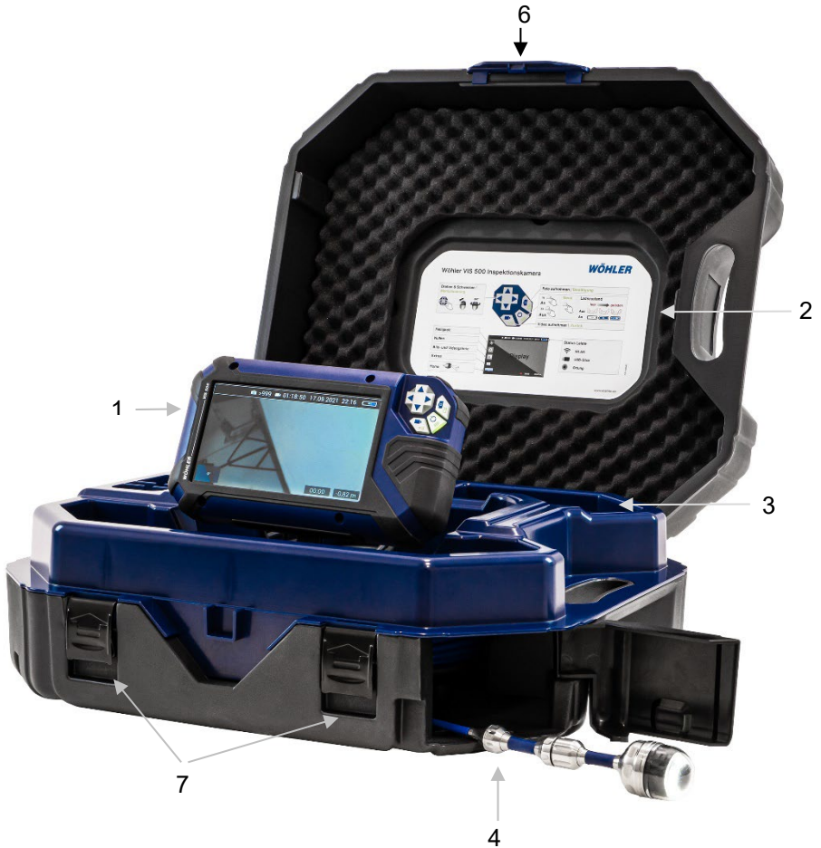
Fig. 6: Wöhler VIS 500 Camera System
