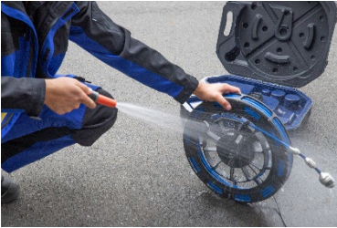
Fig. 57: Cleaning the viper and the rod
